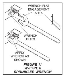
mine the cause of leakage; for example, an improper installation or an ice plug. Close the fire protection system control valve and drain the system before removing the sprinkler.
