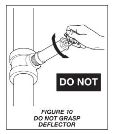
**Note:** If sprinkler removal becomes necessary, remove the sprinkler using the same wrenching method noted above. Sprinkler removal is easier when a non-hardening sealant was used and torque guidelines were followed. After removal, inspect the sprinkler for damage.
