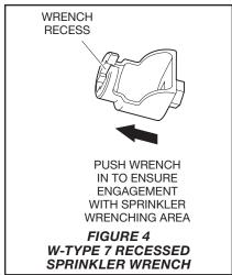
Care must be exercised to avoid damage to the sprinklers before, during, and after installation. Sprinklers damaged by dropping, striking, wrench twist/slippage, or the like, must be replaced. Also, replace any sprinkler that has a cracked bulb or that has lost liquid from its bulb. (Ref. Installation Section).
