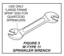
**Step 3.** Tighten the sprinkler into the sprinkler fitting using only the W-Type 11 Sprinkler Wrench (Ref. Figure 3). With reference to Figure 1 or 2, apply the W-Type 11 Sprinkler Wrench is to the wrenching area.
