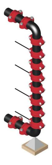
When using flexible couplings, the movement that occurs in long lengths of piping needs to be considered. Each joint can move up to the maximum pipe end separation published. This movement can accumulate and result in the growth of the piping system, for example at the top. Offsets may be necessary.
