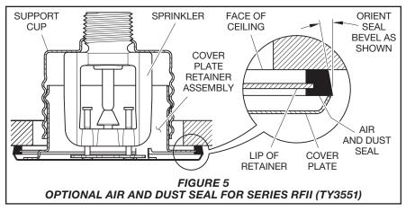
If you must remove a sprinkler, do not reinstall it or a replacement without reinstalling the Cover Plate/Retainer Assembly. If a Cover Plate/Retainer Assembly becomes dislodged during service, replace it immediately.
