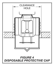
Arms during ceiling installation and/or finish. You can also use the Protective Cap to locate the center of the clearance hole by gently pushing the ceiling material up against the center point of the Protective Cap.
