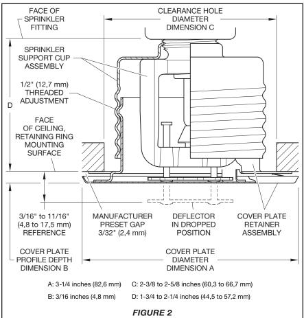
SERIES RFII CONCEALED PENDENT SPRINKLER INSTALLATION DIMENSIONS
