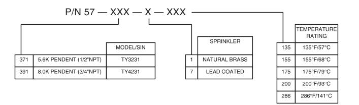
TABLE C PART NUMBER SELECTION SERIES TY-FRB PENDENT SPRINKLERS (MODEL S2 PENDENT SHIELD & O-RING MUST BE SEPARATELY ORDERED)
